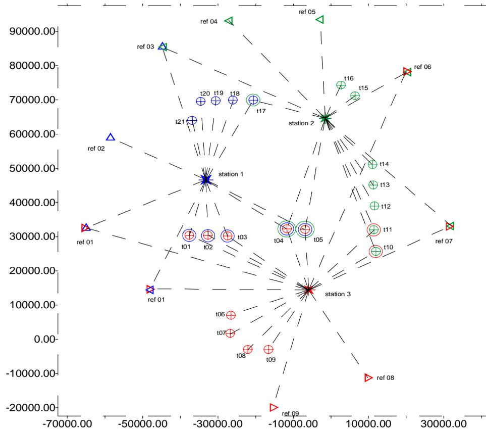
In Amsterdam, the whole monitoring network has been simulated before being set up. There are 23 groups of 2 to 5 total stations.
