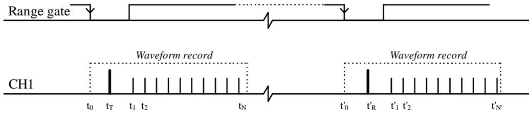
**Figure 2 : Timing diagram of the optically auto-calibrated SLR system of fig. 1.**
