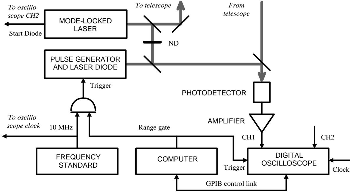
**Figure 1 : Block-diagram of the optically auto-calibrated SLR system with optimum range receiver potential.**
